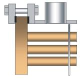
The stationary tube sheet is fastened with bolting between shell flange and front cover flange. Flat gaskets on both sides of the tube sheet seal against water and oil leakage to atmosphere. The floating tube sheet can thermally expand in axial direction. A double rubber packing held in place by a support ring seals on the circumference of the tube sheet against oil getting into the water cycle and vice versa.
