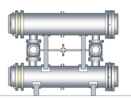
For oil systems with high availability requirements, **OELECHNIK** offers the twin cooler assembly including continuous-flow transfer valves. Each oil cooler is designed to handle 100% oil flow. The flow can be switched from one cooler to the other with the help of two transfer valves connected to shell side oil in- and outlet. Tube side fouling on the oil cooler which is not in operation can be removed without causing any downtime of the system.
