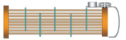
**OELIECHNIK**'s TE MA Type **BET** is only used for even pass numbers on the tube side. In- and outlet connections of tube side are therefore on one side. The integral bonnet has to be removed in order to have access to the tubes on the floating end of the bundle.
