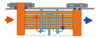
The stationary tube sheet is clamped between shell flange and water bonnet. The floating tube sheet slides in the external seal formed by shell flange and rear bonnet. Regular segmental baffles guide shell side fluid through the shell.
