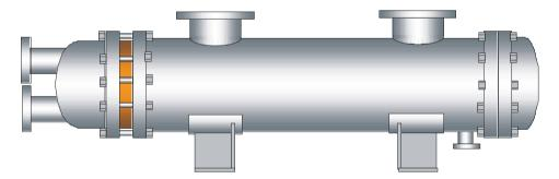
The rear water channel on the floating tube sheet is covered by the rear end bonnet which is bolted to the shell flange. The baffles have a disk and doughnut design. Water is going through the tubes, gas through the shell. The centre of the bundle does not show any tubes which reduces the gas side pressure drop.
