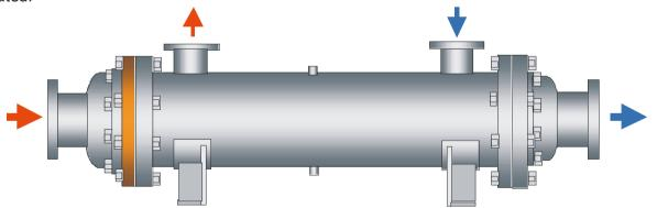
The bolt circle, gasket groove, and inner edge of the floating head bonnet determine the outer tube limit on the tube sheet. Disk and doughnut baffles are used for this design to block the clearance between inside shell diameter and outer tube limit. The rubber packing seals against leakage to atmosphere on the outer edge of the tube sheet. It is held inplace by a packing gland bolted to the shell flange.
